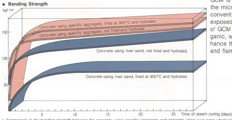
\* Comparison in the bending strength between the concrete using specific aggregate and concrete using river sand which were fired or not fired and hydrated.
